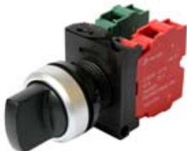
旋钮 |
